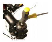
Prior to the final tightening of the screw, rotate the Cycle2Charge to have the USB outlet in the preferred direction.
