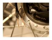
Thread the two twisted wires back into the gray plug and bend the copper wires according to the following picture.
